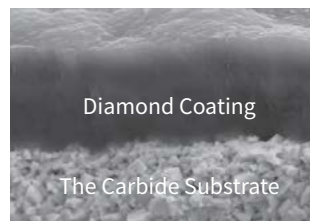
SEM Photograph of Coating
