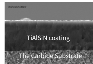
SEM Photograph of Coating
